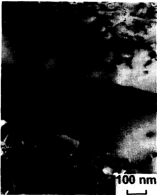
Fig. 8. Transmission electron image illustrating the onset of PFZ formation at grain boundaries.
